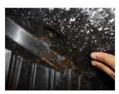
9. Run the light harness (800102-MPX) from driver side to curb side by removing vehicle's front grill.
